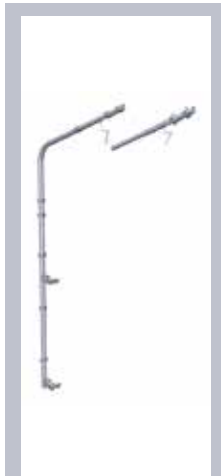
Canopy roof Canopy support - bay width 700-770 mm. Canopy support + 1 extension tube = bay width 1050-1250 mm. Canopy support + 2 extension tubes = bay width 1655 mm
