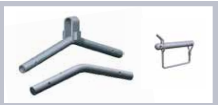
Ridge connector + spring pin The ridge connectors should be fitted using 4 spring pins (12 mm) per connector
