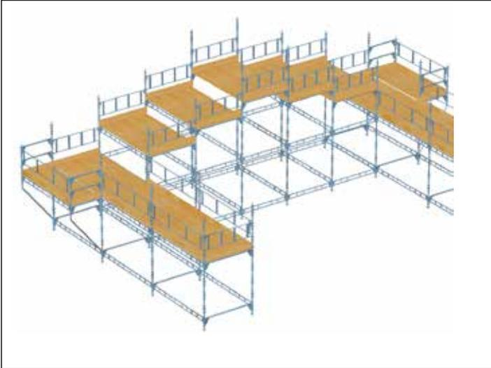
This is a method of erecting a HAKITEC 750 Roof where collective fall prevention is used throughout.
