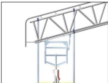
Fix trusses to standards using method specified by the design drawing.
