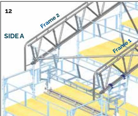
**12.** On frame 1, tension the clamping devices on the beam adapters properly before rolling out.
