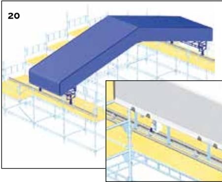
**20.** Release temporary fixings at trusses and rolling gear. Move braking couplers forward along track.
