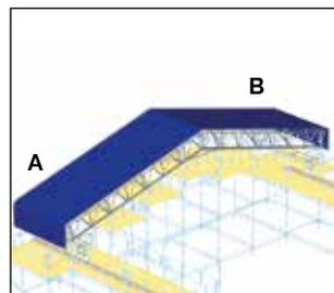
Continue to pull over the sheet until 100 to 300 mm of the sheet remains outside the HAKI Trak tracks on side A.
