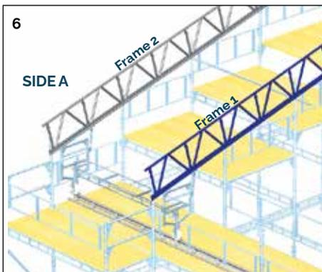
**6.** At the front edge of the gable scaffold, repeat step 3a with truss resting on temporary tubes as above.
