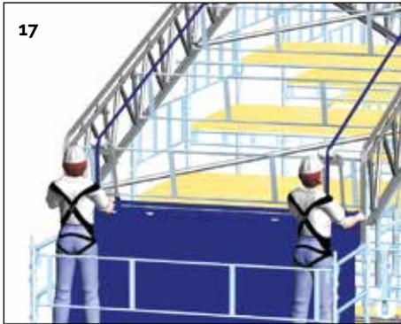
**17.** Carefully pull in the ropes. Make sure that the pulling device wheels are correctly positioned and feed end of sheet into open end of track.
