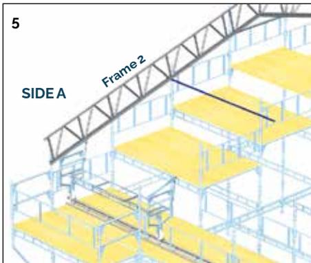
**4.** Loosen the temporary fixing in the ridge, without removing it and allow the complete truss to settle down and thus slide on the beam adapters.
