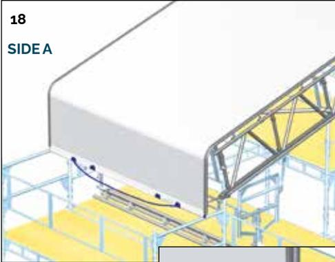
**18.** On side A, push the tension bar through the sheet pocket.
