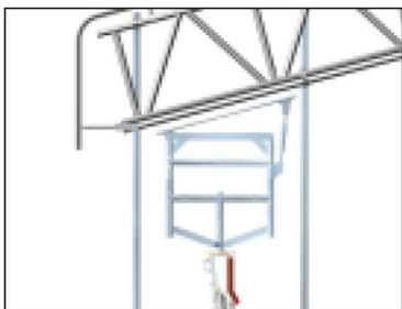
Remove Pin & Chain from Rolling Roof Wheel.
