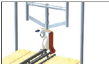
Remove adaptor clamps and wind down the wheel jacks until the beam adaptor is fully clear of the underside of the truss.
