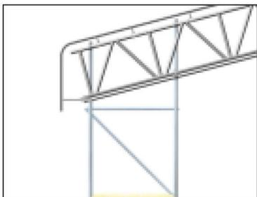
The rolling gear can then be moved away from the underside of the truss. Dismantle and remove. Fit specified Lacing and Bracing.
