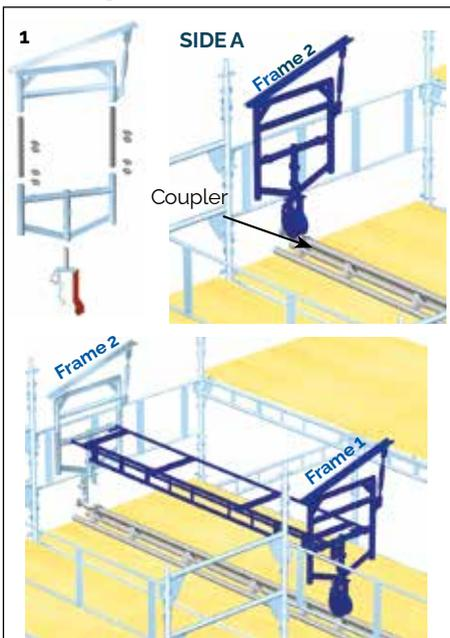
**1.** By frame 2, at the rear of the gable scaffold, place a rolling roof wheel with anti-lift device on the track.
