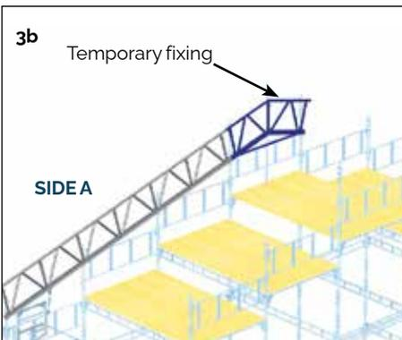
**3b.** Fit the angle frame using two connector tubes and eight 12 mm spring pins.
