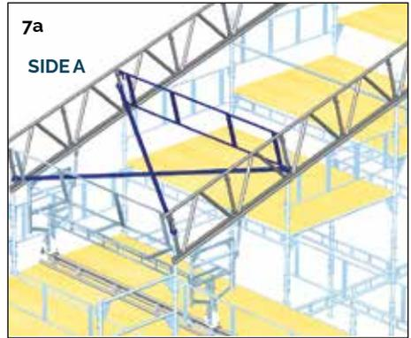
**7.** Fit a guardrail frame vertically in the outermost group of pockets in the eaves in order to obtain the correct distance between the lattice beams.
