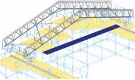
If the design requires knee braces, tie chords etc., a cantilevered platform is provided at an appropriate level throughout the whole gable length.
