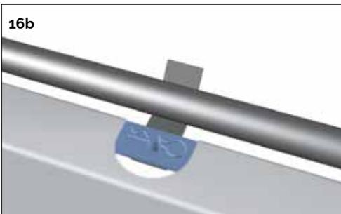
Thread sheeting bar through sheet pocket and attach to pulling device.
