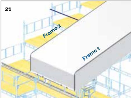
**21.** Fix level horizontal tubes to gable scaffold standards at the underside of frame 2. These will act as a template for subsequent trusses.
