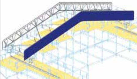
14. Where applicable, check that the pelmet sheet is fitted on frame 1.
