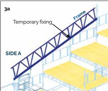
**3a.** Place the first frame on the beam adapter at the correct angle and fix temporarily to the rear of the gable scaffold.
