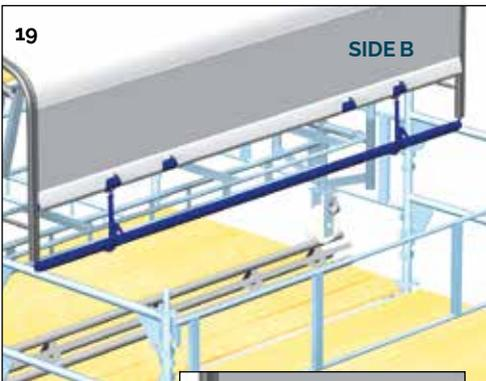
**19.** On side B, remove pulling device and sheeting bar.
