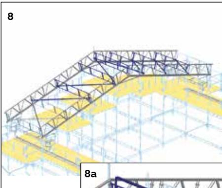
**8.** Work from one side to the other and fit the remaining lattice beams, guardrail frames and plan braces until the frame up to the first bay is finished.
