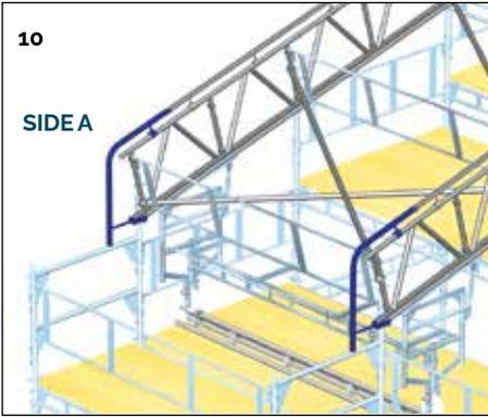
**10.** At eaves fit HAKI Trak end tracks and the track clamp end brackets using 12 mm spring pins.
