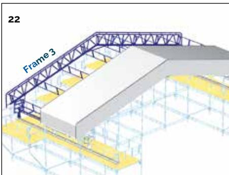
**22.** Repeat steps 6 to 19 for the rest of the roof structure. Only install additional plan bracing as required by the design drawing.
