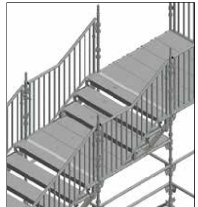
Alt. use of Stair stringer entrance 3 step (7102006) and Stair handrail 1655x500 (7058050).
